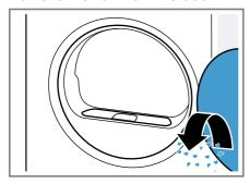
3. Remove the two-part fluff filter.
