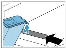
Observe the mark for filling the water tank next to the front opening. If  $\triangle$  does not go out on the display, align the appliance correctly. → "Aligning the appliance", Page 16
