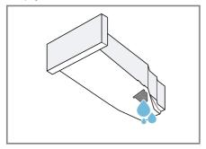
Check the condensation container filter regularly and clean the filter if it is dirty.  $\rightarrow$  *Page 39* Make sure that you insert the condensation container before operating the appliance.  $\rightarrow$  *Page 32*
