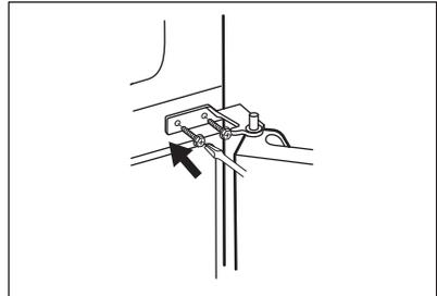
16. Fit the upper hole of the lower door on the middle hinge pin. Tighten the screws.
