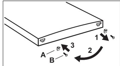
7. Unscrew the screws from the middle hinge. Remove the middle hinge and put it aside together with the screws. Be careful not to lose washers that may stick to the door.
