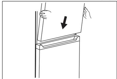
18. Put the upper hinge to the left top side of the appliance. Supporting the door with your hand put the hinge pin into the upper hole of the upper door. Tighten the screws of the upper hinge.
