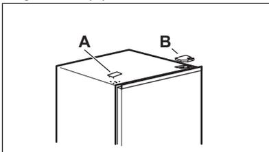
4. Unscrew the screws of the right upper hinge. Support the upper door with your hand. Remove the upper hinge, reverse it, screw the screws and the pin to it. Put
