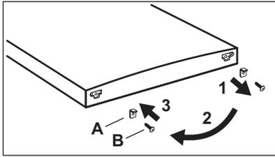
10. Remove the hole cover of the middle hinge and put it in the holes on the opposite side.
