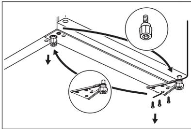
13. Reverse the lower hinge to the other side of the appliance, screw it with screws and install adjustable feet.
