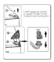
3. Remove screws 1 and hinge 2. Then pass connector 3 through the hole of hinge 2.(Please hold upper door by hand when installing).
