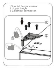
16. Connect electrical connector 1 as shown in the picture, then fix part 2 by screw 3 refer to step 2.
