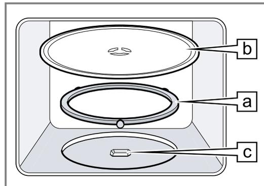
3. Check whether the turntable is correctly engaged.
