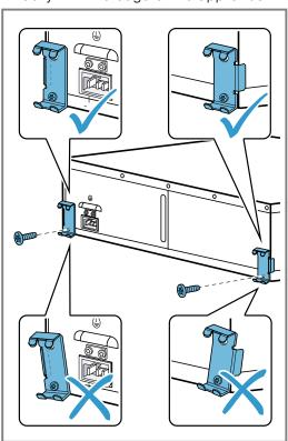
7. Slide the appliance into the fitted unit and check whether the tilt protection engages.
