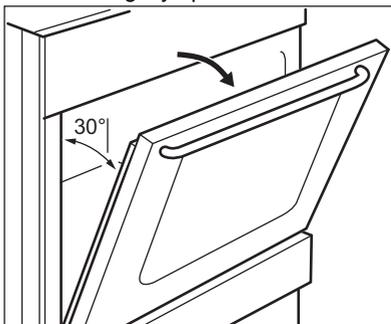
2. Hold the door trim (B) at the top edge of the door on both sides and push inwards to release the clip seal.
