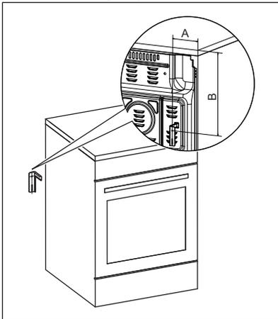
2. You can find the hole on the left side at the back of the appliance. Lift the front of the appliance and put it in the middle of the space between the cupboards. If the space between the bench cupboards is larger than the width of the appliance, you
