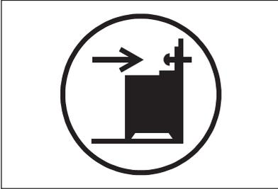
1. Install the anti-tilt protection B - 343 down from the top surface of the appliance and A - 67 mm from the side of the appliance into the circular hole on a bracket. Screw it into the solid material or use applicable reinforcement (wall).
