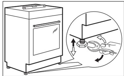
Use small feet on the bottom of appliance to set the appliance top surface level with other surfaces.
