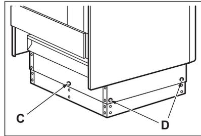
6. Push the plinth in to the required height setting: 923, 898 or 858 mm.
