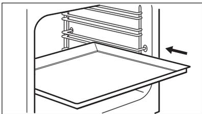
Push the tray or deep pan between the guide bars of the shelf support. Make sure it does not touch the back wall of the oven.
