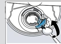
5. Lift the pump cover inwards at an angle and remove.
