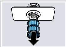
4. Press the locking catches ① together and lift the coarse filter out ②.
